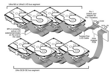
Figure 3. Cable connections and external termination
